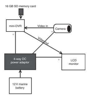
**Fig. 1.** Schematic design for using the underwater video camera (UVC) system to sample fish in dense submersed vegetation. A 12-V DC marine battery powers the system. Power adaptor connections to the digital video recorder (DVR), UVC, and video monitor are indicated with a + symbol. The 16 gigabyte memory card is used to store video recordings from the DVR. Video cables connect the camera to the DVR, and connect the DVR to the video monitor.
