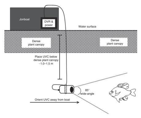
Fig. 2. Diagram for underwater camera deployment to sample fish in dense aquatic plants.
